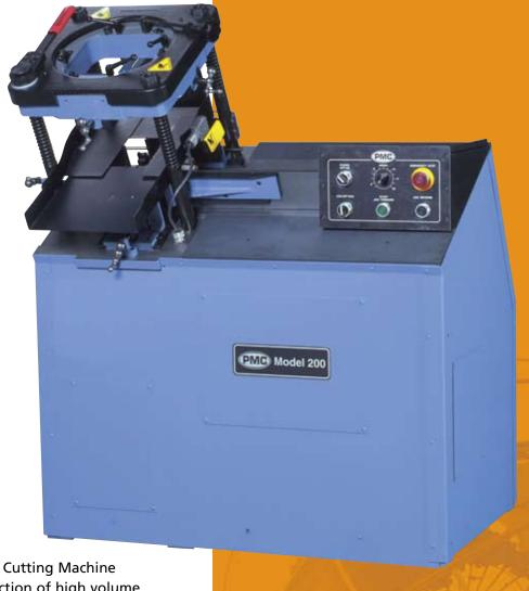
The PMC **Model 200** Die Cutting Machine revolutionized the production of high volume accurate labels. With a variable speed electronic drive and a trouble-free mechanical disappearing shuttle, the **Model 200** doubles the production of ordinary die cutting machines. The **Model 200** can be used as a stand-alone manual machine or in conjunction with a Bander, Feed Table or Strip Cutter to form an automated production line.
